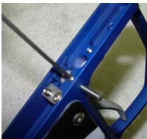
To remove the trigger, loosen the setscrew holding the trigger pin with an Allen wrench. This must be done with the body off the trigger frame. Removal of the trigger may cause the trigger spring to drop out and become lost. It is best to remove the gun body and ram body completely from the trigger grip frame. Then remove the trigger spring holder and the spring before removing the trigger pin.
