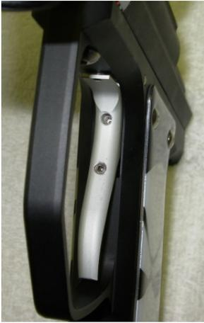
There are four adjustments. Two are adjusted on the front of the trigger. The trigger contact point is the top set screw. Turning the screw clockwise makes the contact point sooner, counterclockwise to make the contact later.
