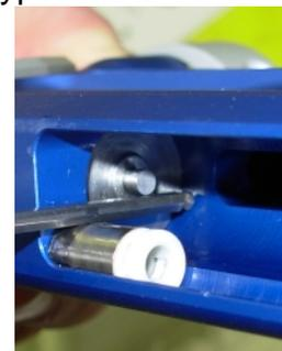
With the setscrew to the Cup Seal Valve in place you can see that the threads holding the setscrew are missing on the sides. This is because of the oval cut made to match the cut in the top of the cup seal for the Sweep airflow.
