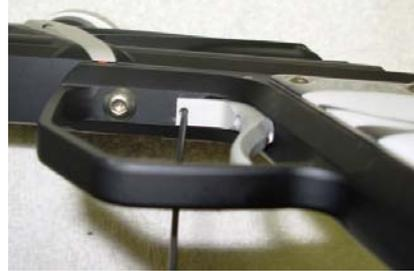
The setscrew to adjust the trigger return travel can be adjusted by fitting an Allen wrench through a hole in the trigger lever on the under side of the trigger guard. Clockwise increases travel – counterclockwise limits travel.
