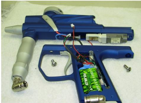
The marker components are visible. The valve pin assembly is easily viewed, as is the hose and the hose fittings. Hose fitting are quick release type. To remove the ram – without pressure in the hose – push the fitting release toward the fitting body, pull on the ram body; the hose will easily slide out of the fitting.
