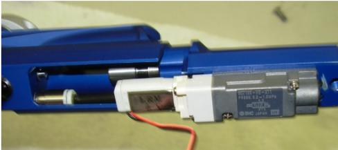
Slide the ram into the gun body while sliding the hose into the fitting. The gun now consists of two half's: the gun body with the ram, and the Trigger frame.
