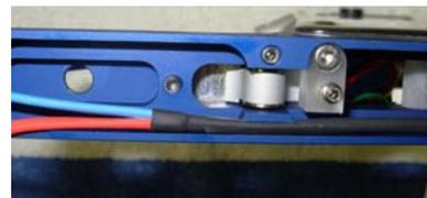
Do not pull too tightly on the eye wire when you tuck them into the groove in the trigger frame as this can pull the wires down inside the eye covers and misalign the eyes. This is also why you have ***aligned the trigger frame about a half and inch forward in relationship to the gun body,***
